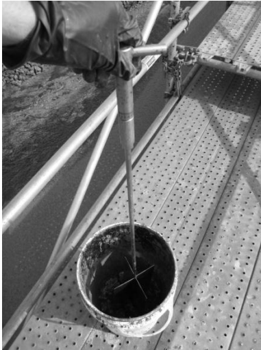
Figure 4. Manual vane for rheological field monitoring. Vane diameter is 150 mm.
