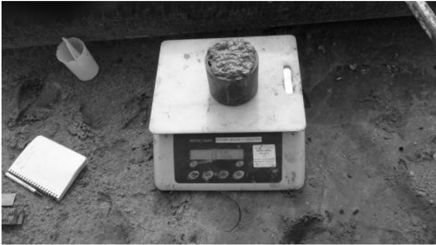
Figure 4. Simple, modified slump test set-up for field rheology. Balance used for bulk density determination.
