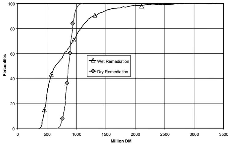
Fig. 1 Equivalent Costs for the Wet and Dry Tailings Reclamation of the Helmsdorf pond.
